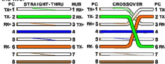
To easily tell if you have a crossover or not, simply look at the two ends side by side. If all the pins, 1 through 8 on both ends are all the same color in the same order, you have a straight-through cable. If pins 1, 3 and 2, 6 are swapped you have a crossover cable. Notice the TX, RX as well. This shows why in pc to pc connections a crossover is required. Otherwise one pc will be transmitting over the same wire the other pc is trying to transmit on.
